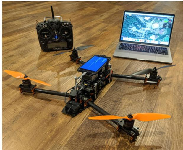
FIGURE 16. DRONE ASSEMBLY WITH MOBILE DEVICE
